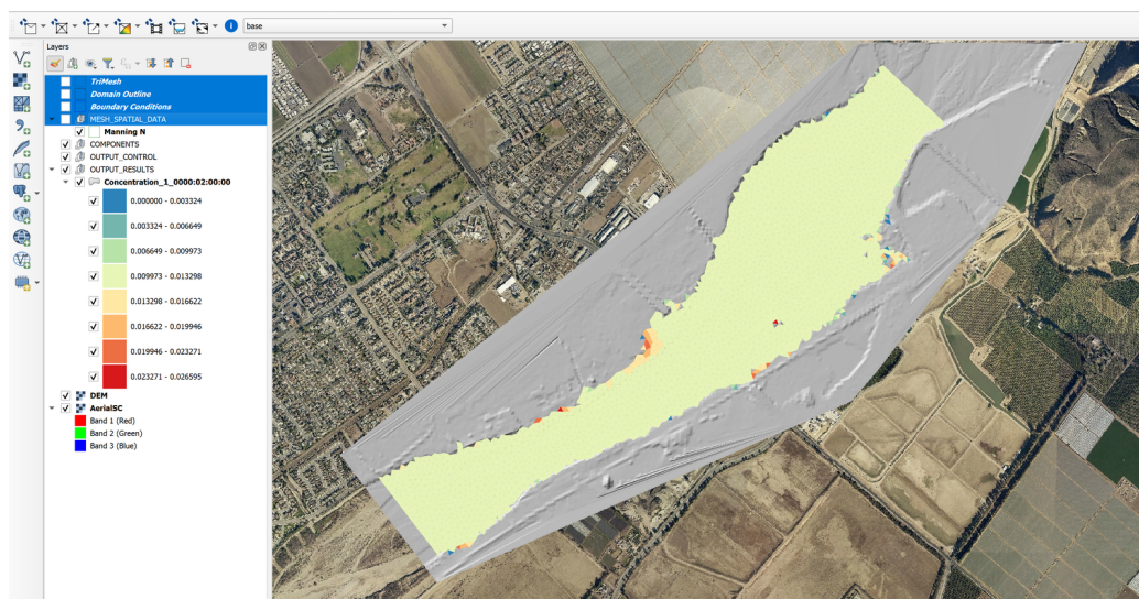
Figure 10.4 – Map of suspended sediment concentration for the last time step.
